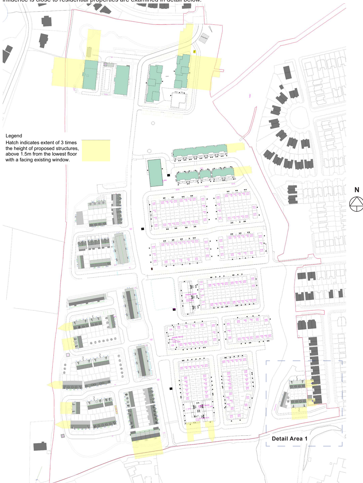
Figure 2: Proposed site plan showing the zone of influence from the proposed building and direction of the window wall of neighbouring residential properties.
